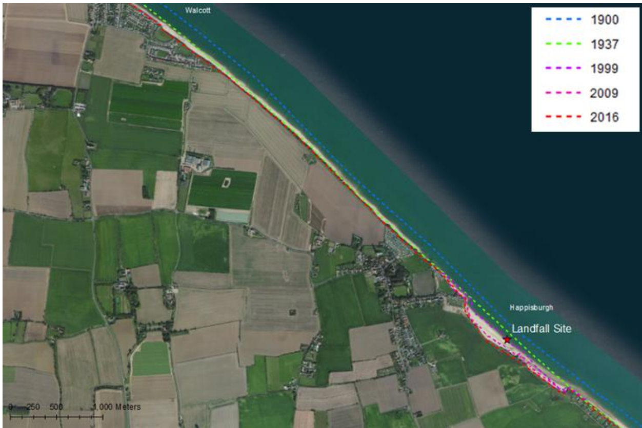
Figure 2-4: Cliff erosion between Happisburgh and Cart Gap
